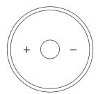
Make sure F1s is unlocked by pressing and holding the + and - buttons together for 3 seconds until the light turns on.
