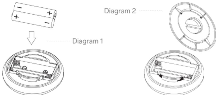
Once in place, insert the plastic key in the cover's slot and do a 10 degree twist clockwise to lock shut. To open, always use the key and make a 10 degree turn counterclockwise before replacing the batteries - using other tools such as coins may damage the surface of the remote (see Diagram 3).
